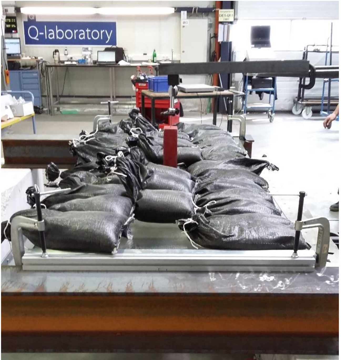
Typical arrangement for application of uniformly distributed load applied to the barrier system
