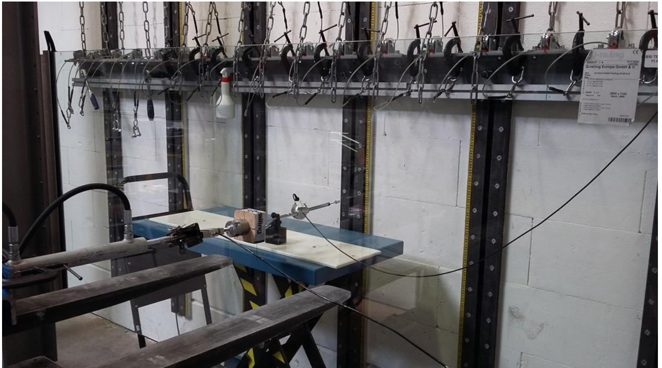
Typical arrangement for application of point load to the centre of the barrier system
