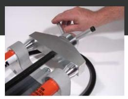
Attach the terminal to the attachment fixture on the drawbar, and adjust the length so the roller dies meet the terminal shank at desired position.
