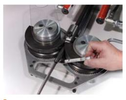
Apply just enough hydraulic pressure so that the roller dies holds the terminal firmly. Then mark and insert the cable into the bottom of the terminal throat.
