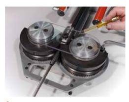
4 Move the transparent protective shield into position. Apply hydraulic pressure to draw the terminal between the roller dies.
