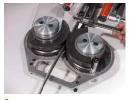
• Measure the diameter of the terminal after swaging, and compare with the swage dimensions list.
