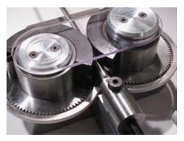
**5** When the roller dies rotate, they will press the terminal shank onto the wire rope.
