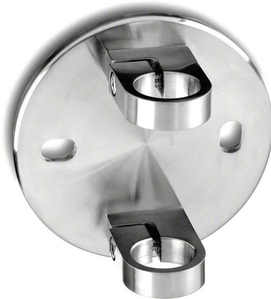
The circular wall mount bracket is a simple, elegant system used to attach your balustrade posts to a wall or other flat surface, easily mounted using two stainless steel wall anchors. It features two elongated fixing holes to allow for precise placement and final angle adjustment. You can choose between either a 45mm or 60mm stand off from the wall surface.
