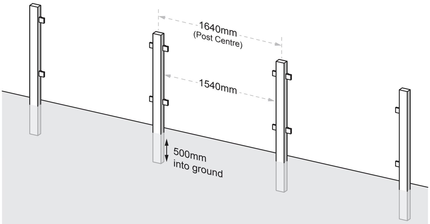
\*These measurements allow for a 20mm gap each side between the post and the panel, which is the depth of the internal section of the clamp.
