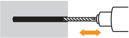
Drill pilot holes for the wood screw thread vine eye bolts.
