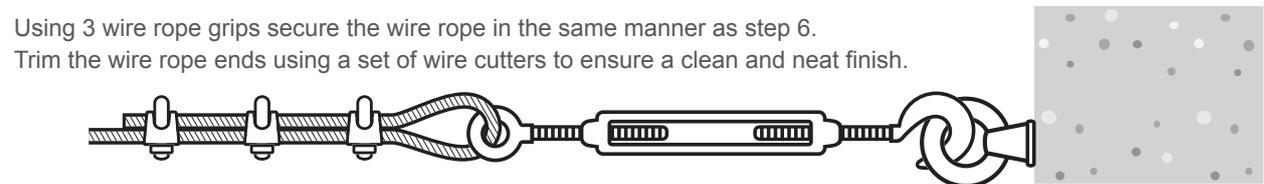
Using 3 wire rope grips secure the wire rope in the same manner as step 6.
