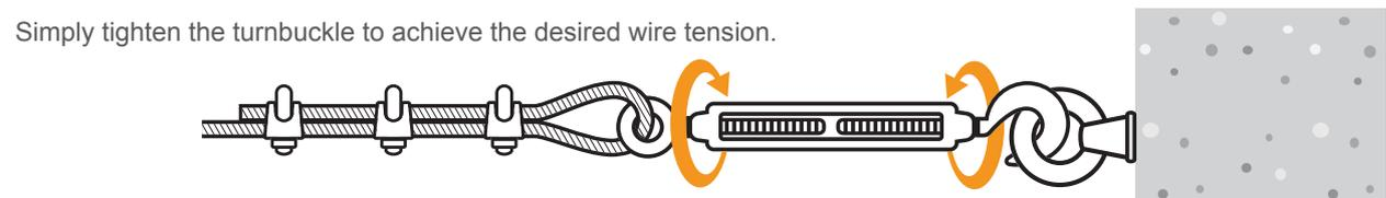
Simply tighten the turnbuckle to achieve the desired wire tension.
