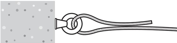
We do not recommend cutting your wire cable to length at this point, as it can be trimmed to the correct length later on - Simply thread one end of the cable through the eye of your first eye bolt bringing it back on itself.
