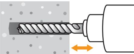
Drill your fixing holes and ensure that the holes are free from dust and debris. We recommend using a small brush and/or an air pump to perform this action.
