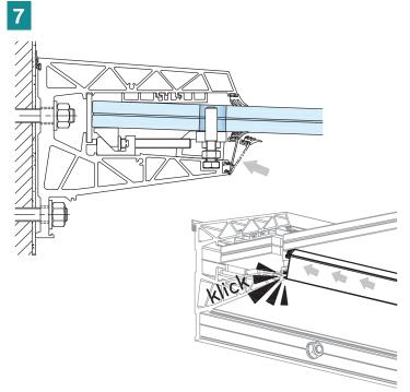
Set the profile cover incl. seal on the base profile and press it into the base profile until it clicks into place.
