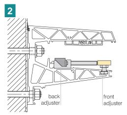
Insert the upper compensation profile and the adjusters (front and back) into the base profile. The number of adjusters varies depending on the profile length.
