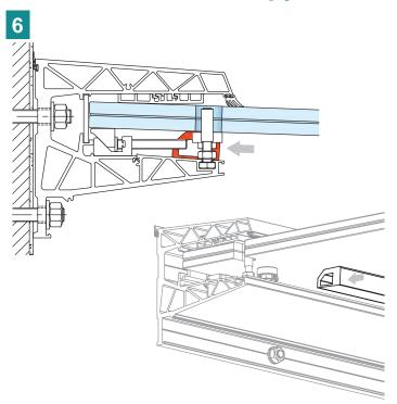
Press the clamping profiles between the glass and the base profile. The number of clamping profiles varies depending on the profile length. Figure C.
