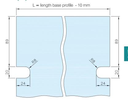
We recommend the use of tempered and laminated glass 10+10+1.52 SG (rigid plastic film - e.g. SentryGlas®) for optimum canopy system stability.
