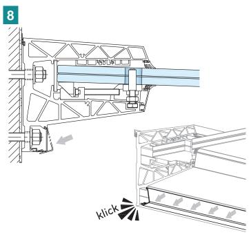
Set the screw cover on the base profile and press it in until it clicks into place. Alternatively, and if there is enough space, the screw cover profile can also be slide into the side of the base profile.
