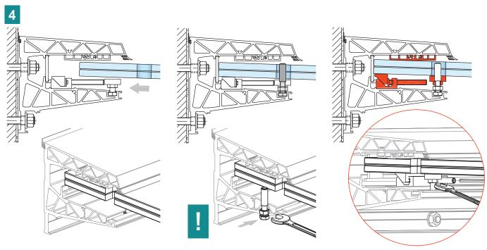
Glass installation: Guide the glass between the adjusters and the compensation profile. The glass must touch the rear spacer plates. Then the glass must be brought to the upper compensation profile with the adjusters. ATTENTION: To secure the glass, immediately insert the safety pin screws on both sides of the profile and secure them with the nuts (the safety pins must be located inside the glass cut outs). The decline of the glass can then be adjusted with the front and rear adjusters.
