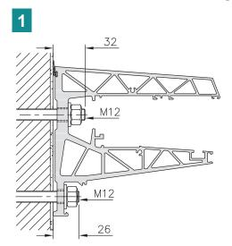
Fasten the base profile (incl. gaskets) to the wall with statically suitable fixing anchors\*. All mounting holes must be used. May use the profile as drilling template.
