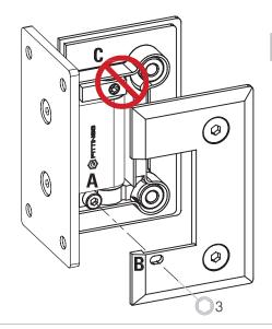
Adjustment of the closed position (0-point): After mounting the glass door, the final position of the door can be adjusted. Loose the screw A (through the opening in the clamping plate B) and align the door as desired. Then tighten screw A again. The screw C shown above must not be loosened.
