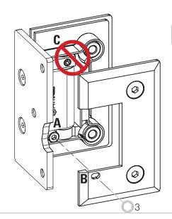
Adjustment of the closed position (0-point): After mounting the glass door, the final position of the door can be adjusted. Loose the screw A (through the opening in the clamping plate B) and align the door as desired. Then tighten screw A again. The screw C shown above must not be loosened.
