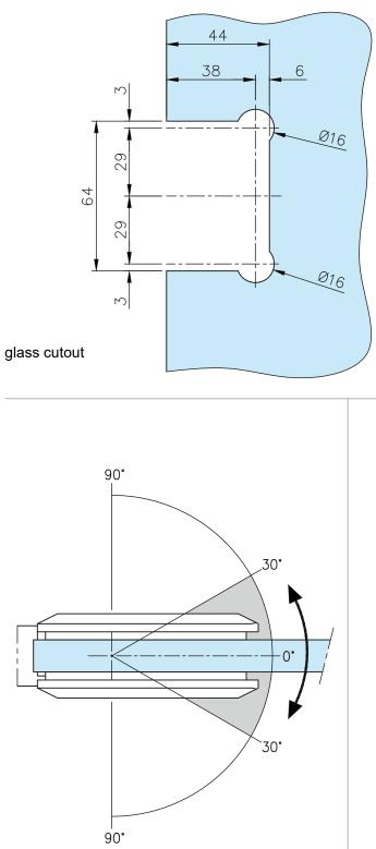
automatic closing action from 30° "Zero point" (0° - closing) adjustable
