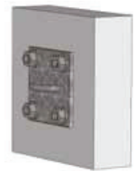
Step 4: Screw the washers and bolts and tighten them onto the wall bracket
