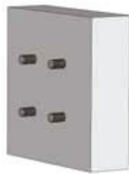
Step 2: Insert M10 bolts anchors into the concrete wall. Bolts are not supplied. Be sure to follow the manufacturer's installation recommendations.
