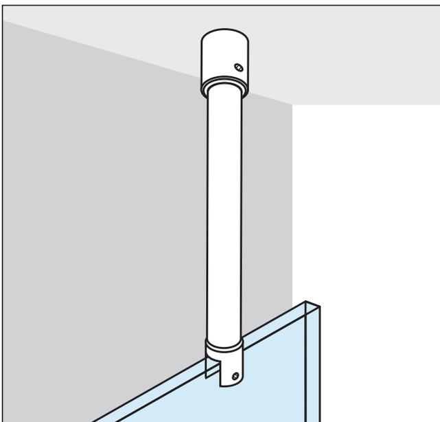
You can use Stainless Steel Adhesive (not included) to fix Tube Insert Clamp in place, although this is not essential, as end fitting is a tight fit and will be held firmly in position by tension between glass and ceiling fitting.
